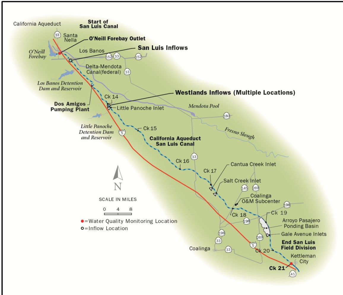
Figure 14-19. Location of Non-Project Inflows in the San Luis Canal Reach of the California Aqueduct
